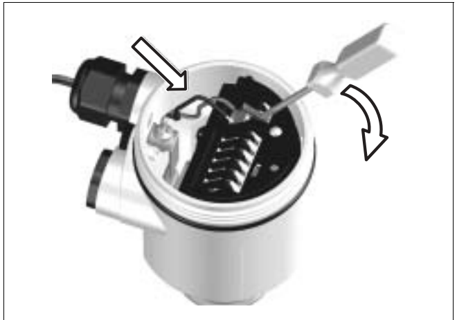
Fig. 5: Connection steps 5 and 6
