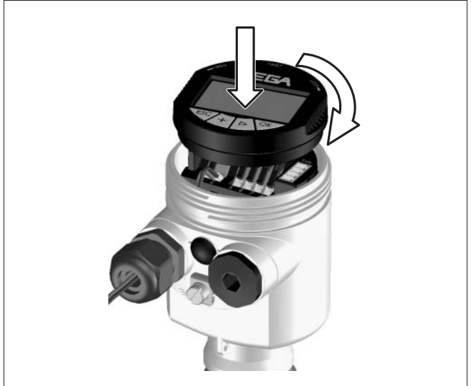
Fig. 14: Installation of the indicating and adjustment module
