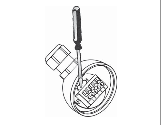
Fig. 10: Adjustment zero and span
