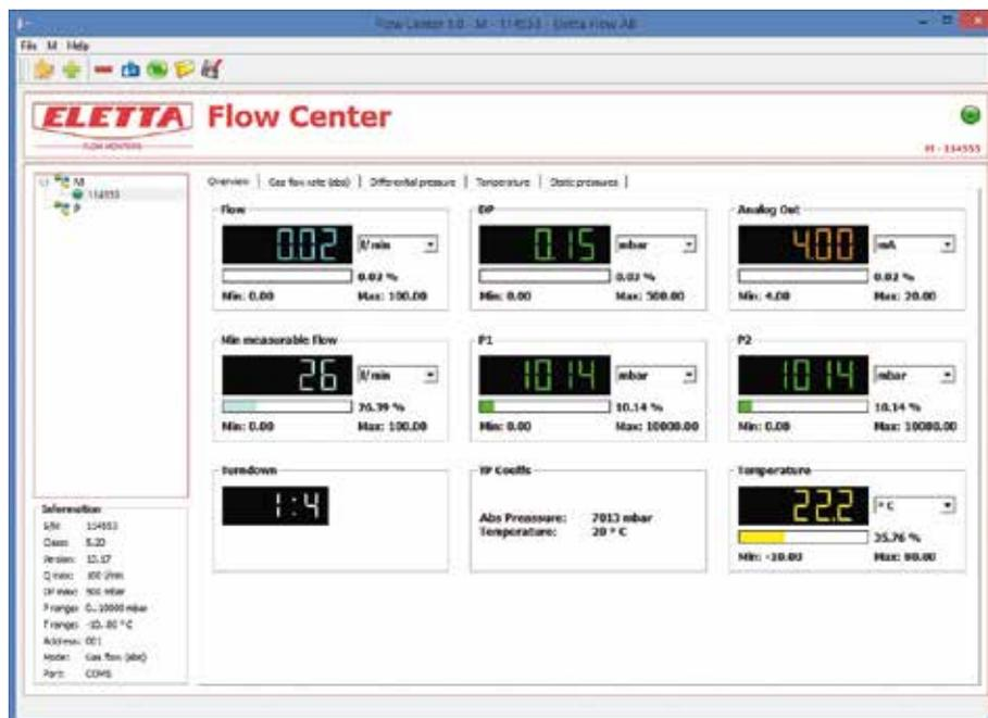
*This picture shows the software's interface. The Overview tab gives a clear overview of all parameters in real time.*
